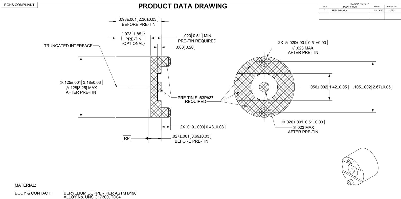
**INSULATOR:** PEEK 1000 PER ASTM D6262
